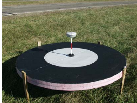
Figure 2. LiDAR target fabricated by the Ohio Department of Transportation
